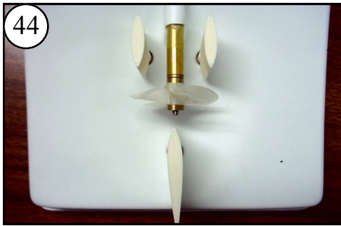
44 Check the Rudder and Flankers to see that all are parallel to the Stern Tube.
