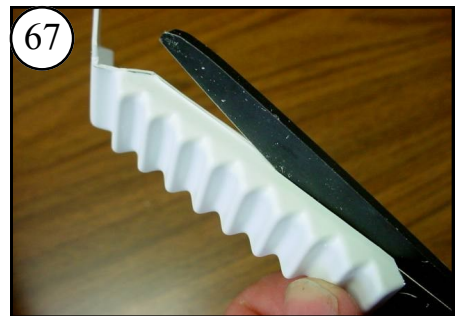
67 After rough-cutting, trim the sides of the stairs with scissors so they are flat. Trim the bottom step so its height is equal to the other steps.
