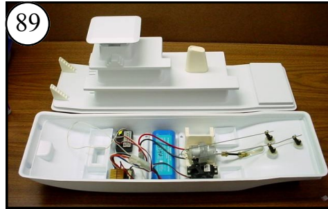
89 Do a final operational check before gluing the Deck to the Hull.
