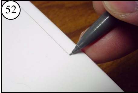
52 The Deck and Hatch openings have a recessed edge that is already marked with a pencil for trimming.
