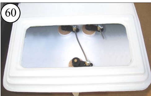
60 Install the set screws for the rudder arms so they can be reached from the hatch. Flankers on the rear (stern) side and rudders on the front (bow) side.
