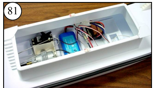
81 Use 6 small pieces of Velcro to secure the 2nd Deck to the Deck. The two pieces at the center will help prevent sag in the 2nd Deck.
