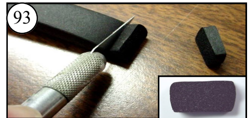
93 Pads for the Push Knees are cut by pressing a hobby knife or razor straight down through it. One side is slightly wider than the other. (Top of inset photo) Glue wider side to Push Knee.
