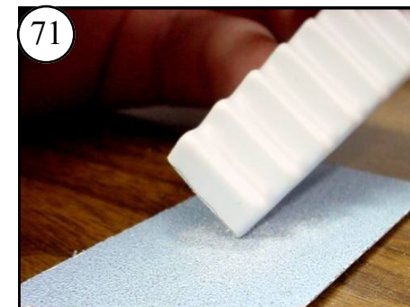
71 Round the bottom corner to conform to the curve at the base of the Cabin.
