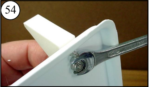
54 Attach the Tow Knees with the galvanized steel nylon locknuts. Tighten with a 5/16" wrench. If they are not square to the front of the deck, adjust the holes with your drill or hobby knife.
