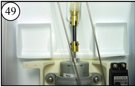
49 The rear Ballast Trays sit on either side of the Stern Tube as shown. Later, they can be attached with a small piece of Velcro for easy removal and adjustment.
