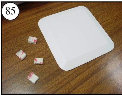
85 Trim the Roof and cut 4 small 1/4" pieces of Velcro.
