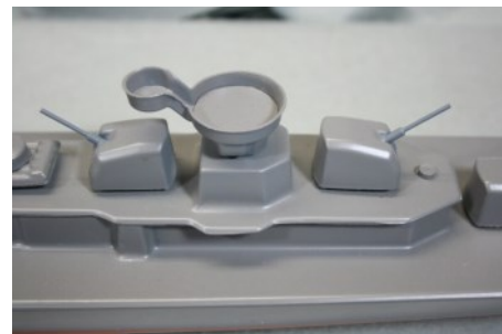
Early Fletchers had an AA gun nount with a rangefinder mount next to it. Later versions had just the gun mount.
