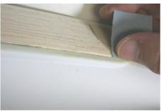
Leading edge before and after. Above the bilge keels, use the edge of the sandpaper to put a small bevel along the bottom edge of the balsa. The taper will help the balsa stay secured to the hull.
