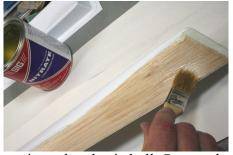
Work a thin layer of dope into the balsa to include the tapered edges. OK to get it on the plastic hull. Start and one end and work along. Don't try to wet the whole length. The dope dries too fast. One coat each side.
