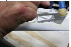
The coating does not have to be thick or lumpy. Coat both pieces of balsa then roll adhesive onto both sides of the hull over the same areas. Start at the front and work rearward. Don't try to roll the whole length at once.
