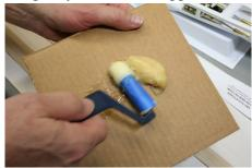
Gel cement is a little less runny and stringy than normal liquid. Put on cardboard and load the roller with glue. 1
