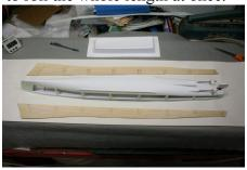
It is OK if you go further on the hull than the edge of the balsa. Beauty is not a priority. Let dry for 10 to 15 minutes. Roll up a plastic bag to keep your roller from drying. Apply a 2nd coat to the balsa sides and to the hull. Let dry at least 15 to 20 minutes according to the can's instructions. It will be dry to the touch.
