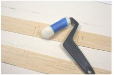
Silkspan side up, lay the two pieces next to each other and transfer the rib marks. A small mini-paint roller works great for contact cement. Tightly wrapping masking tape around it will give you a narrow applicator.
