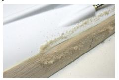
At the stern, the balsa will be sticking up from the hull a little. Sand downward until you reach the point where the balsa is bonded to the hull plastic. Then, put a taper along the side of the balsa in this area.
