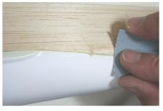
Once the balsa is stuck tight, take the sanding board and put a slight taper along the top of the balsa sides just until you see the white edge of the hull styrene (arrow) exposed by the sandpaper. On the bottom edge, hold the small piece of sandpaper in a dish shape to put a taper on the bottom edges of the balsa strips.
