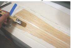
Lightly wipe with fine sandpaper to knock off any bits. Lay a piece of silkspan over the two sides. Securing with tape at each end will stretch out wrinkles and make it easier to brush on one coat of dope over the silkspan. The dope will penetrate the silkspan and bond it to the dried first coat of dope to strengthen the balsa.
