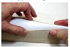
Once the top is bonded, turn the hull over and press along the bottom to bond the balsa to the hull. It is fragile.
