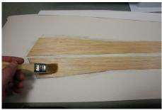
Protect your work surface with a layer of paper. Trace the pattern twice on 1/32-inch balsa. Cut out the two pieces with a hobby knife. Lay out the two sides as shown. Brush one coat of Dope to one side and let dry 30 minutes.
