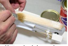
Holding the silkspan at the stern, evenly overlapping the balsa at the top and bottom, brush dope on the silkspan. It will soak through and bond the silkspan to the balsa and hull. Work along the hull, holding the silkspan in a slight tension and keeping it aligned as you brush the dope on to seal all areas.
