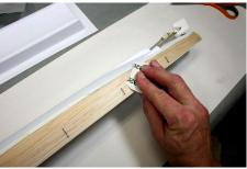
While the hull is drying, use the balsa pattern to mark and cut two pieces of silkspan with the cut marks about 1/4" larger than the pattern on all sides. When dry, lightly wipe the surface with fine sandpaper to remove any bits.
