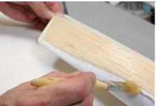
The dotted lines show the edge of the silkspan. Use the brush or your finger to press out any gaps or bubbles along the edges. Once this side is dry to the touch, cover the other side with the other piece of silkspan. Once dry, use a hobby knife to trim off any excess silkspan sticking up above the top side of the deck.
