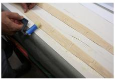
Use the untaped end as a narrow roller. Start at one end and work an even coat of contact cement about 3/8-inch wide around the edges, at each rib and larger areas at each end on the SilkSpan covered sides of the balsa.
