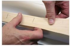
Continue to work and press along the top to each end. Repeat for the other side. Gently pull and align the balsa.
