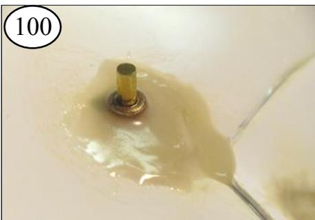
100 Mix the last batch of filled epoxy. Make sure the third layer is still lower than the top of the bearing.
