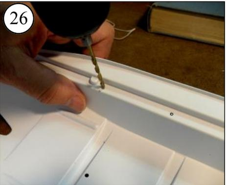
26 Drill 3/32 inch holes at the 4 marked Servo Tray holes.
