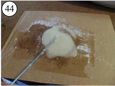
44 Mix the epoxy and add filler. Find the Epoxy Brush.
