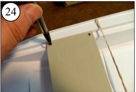
24 With the Servo Tray slid against the raised bumps on the liner, mark the 4 holes with a pencil.
