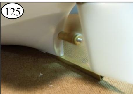
125 Check the direction of the prop. Going forward, it should be turning counter-clockwise as seen from the back.
