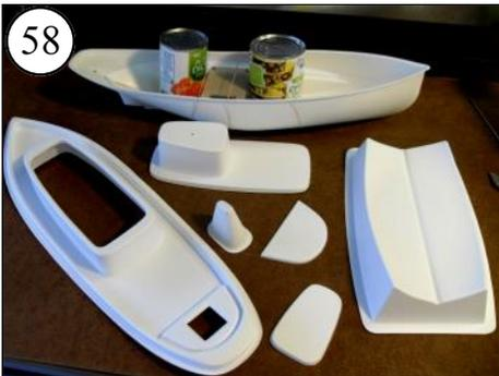
58 All trimmed. The hull should be set by now. Check the mixing board to make sure.
