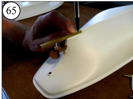
65 Place the Skeg on the hull, aligned with the keel (bottom board) of the hull. Mark ONLY the end screw hole.
