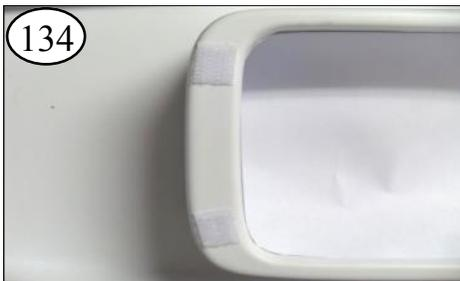
134 Stick the Hook & Loop squares on the front and rear of the Cabin as shown. Peel tape. Set Pilot House on Cabin to adhere the Loop to the Pilot house. Remove Pilot House and press the Hook & Loop to set the adhesive.
