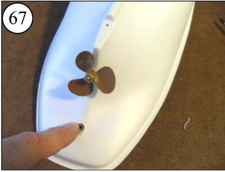
67 Press the Rudder Bearing into the 1/4 inch hole.
