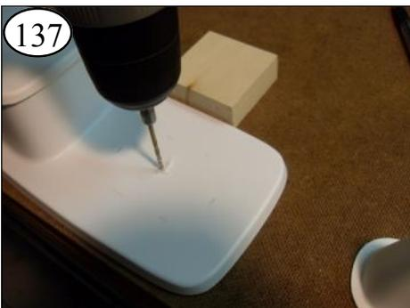
137 Drill a small vent hole in the center of the marked area.
