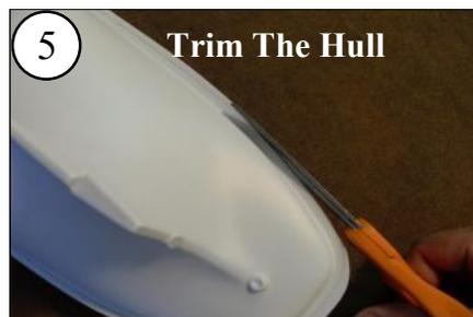
Trim the Hull along the marked line on it’s underside. The plastic is thick for a stronger hull. Use sharp scissors!
