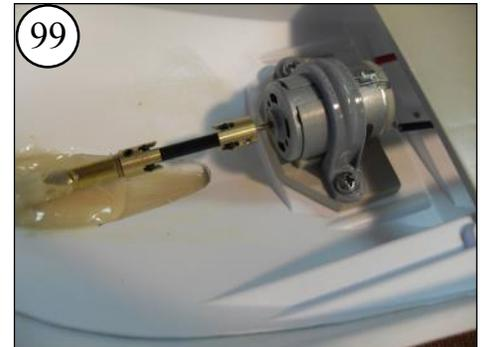
99 Test-Fit the motor to the Stern Tube with the Dogbone between the Coupling Ends.
