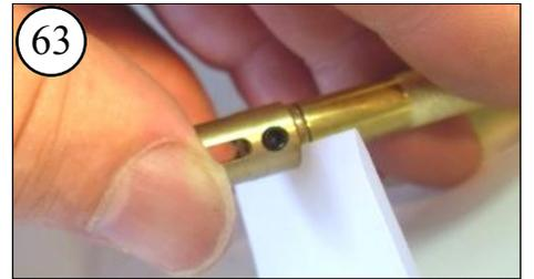
63 Fold a piece of paper and use it as a spacer between the coupling end and the stern tube. Tighten the two set screws and remove the paper. This should leave a small gap there.
