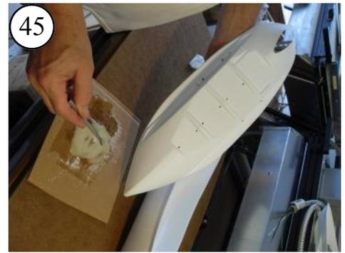
45 Holding the Liner, apply the epoxy by lightly dabbing the sanded areas.
