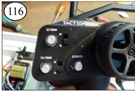
116 Connect the ESC, battery, & servos from the instructions for your electronics. Set transmitter steering adjustments to neutral.
