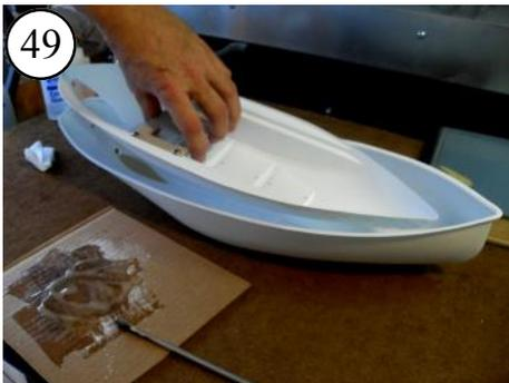
49 Insert bow-first, trying to avoid touching the sides of the Hull with the Hull Liner.
