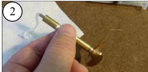
Push the Prop Shaft into the stern tube. This will push out the excess grease. Wipe off the excess with a paper towel. Be careful to keep any grease off of the brass Stern Tube.
