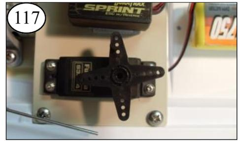
117 Turn on the Transmitter first, then the receiver using the switch on the Electronic Speed Control. In this case, the servo horn is angled.
