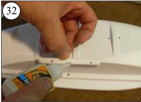
32 Apply Medium CA (super glue) to one strip. Hold the strip against the underside of the rail with the holes aligned.
