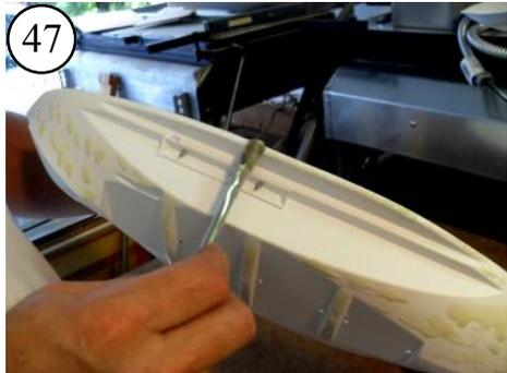
47 Dab along the sharp edges. 30-minute epoxy can gel in 10 min.
