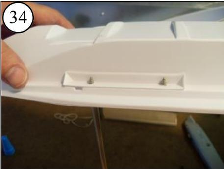
34 The screws should pull the Reinforcing Strip tight against the Hull Liner.
