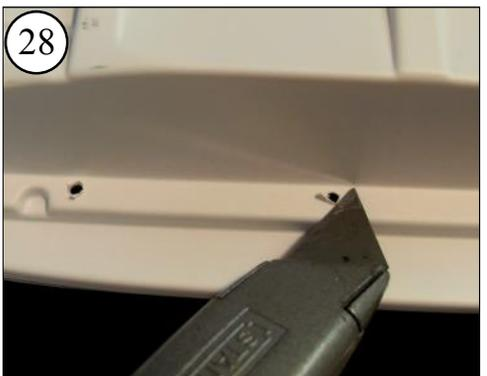
28 Trim any bits from the underside of the drilled holes.
