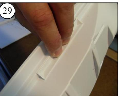
29 Hole the Reinforcing Strip under the tray mount holes.
