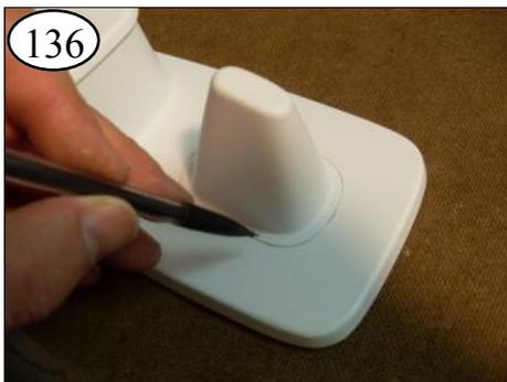
136 Center the Stack on the deck of the Pilot House. Lightly mark the location in pencil.
