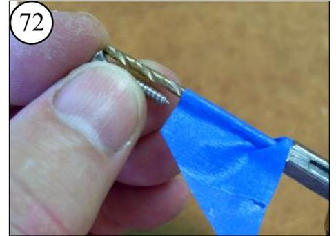
72 Using a Skeg screw as a guide, wrap a piece of tape on the drill to make a depth gauge.
