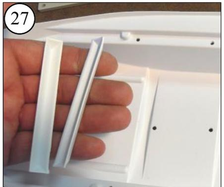
27 These are the Servo Tray Screw Reinforcing Strips. They provide a better anchor for the screw threads.
