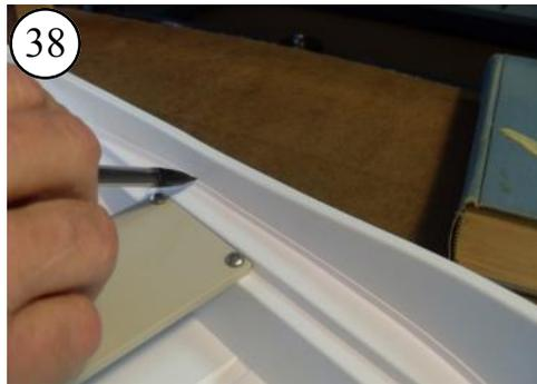
38 Set the Hull Liner into the Hull. Use a pencil to lightly mark the hull along the top of the Liner.
