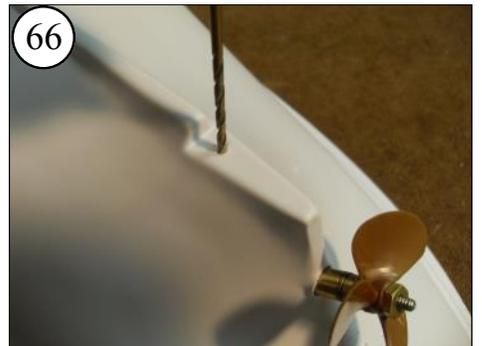
66 Use a 3/32 inch drill to drill a straight hole through the Hull and Skeg Reinforcement.
