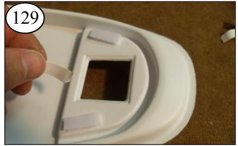
129 Stick the hook side to the hatch as shown, away from the opening. Put the fuzzy loop side on top and remove paper from the adhesive.
