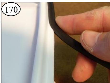
170 This bend will help the Rub Rail open and engage the flange of the hull. No need to glue it. It will stay in place.
