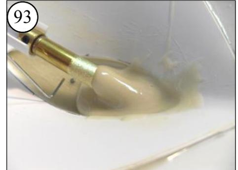
93 Put the filled epoxy over the Prop Shaft Assembly where it comes through the Hull.
