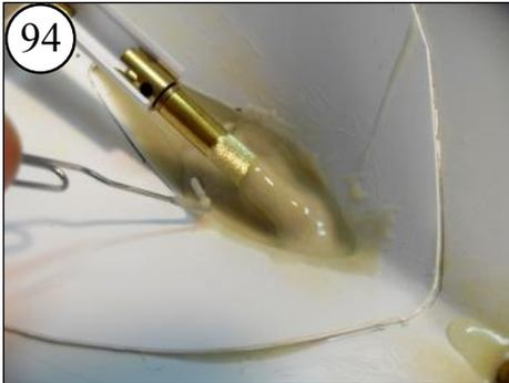
94 Push the epoxy under the Prop Shaft Assembly to eliminate any air bubbles under it.
