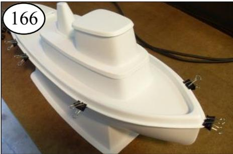
166 Notice the clamps are not jammed against the hull. They are centered on the flange. A few final clamps may need to stay on longer to bond.
