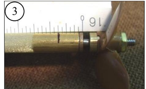
Put a mark on the Stern Tube about  $3/8^{\text{th}}$ s of an inch from the end of the bearing.
