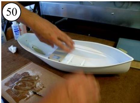
50 Press into place. If the sides of the Hull are not making good contact with the sides of the Liner, add rubber bands.
