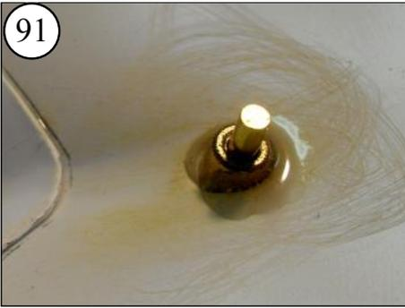
91 Just enough to encircle the bearing and fill the narrow gap between the bearing and the Hull Liner.
