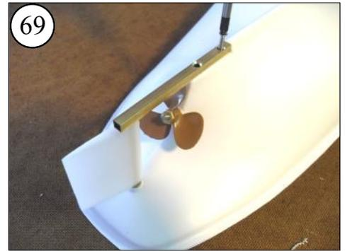
69 Slip the Skeg onto the rudder and attach the bow-end screw into the Skeg. Just snug the screw for now.
