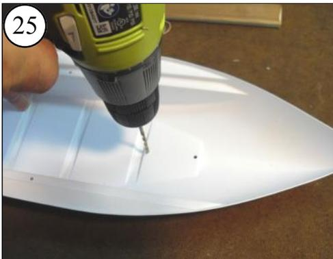
25 Drill 1/8 inch vent holes into the liner on each side of the floor ribs as shown.
