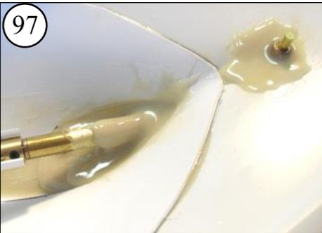
97 Mix a smaller batch of filled epoxy. Carefully apply a layer around the rudder bearing & put the rest over the Prop Shaft Assembly as shown.
