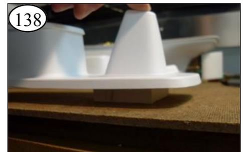
138 Lightly sand the underside of the stack and apply CA. Press 40 seconds onto the Pilot House deck supported by the wood block.
