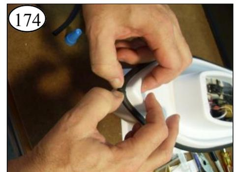
174 Hold tight for one minute. Check under the glued ends and if not together, hold that spot too. **18**
