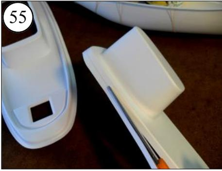
Cut curves by taking shorter snips. If the edge is uneven, you can sand the cut edge.
