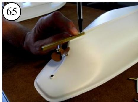
Place the Skeg on the hull, aligned with the keel (bottom board) of the hull. Mark ONLY the end screw hole.
