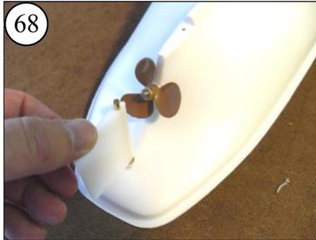
68 Insert the longer brass rod of the rudder into the bearing.
