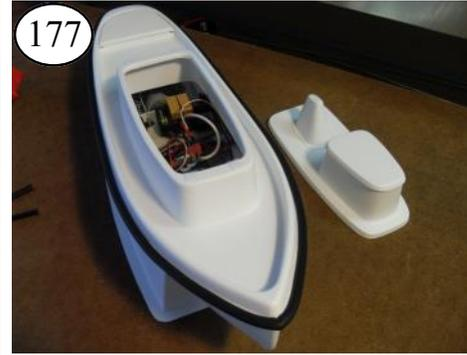
Re-install the Rub Rail starting with the (front) bow end and work backwards.
