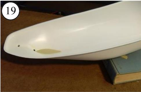
19 Tilt up the hull with a book to keep the epoxy in place as it cures.
