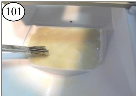
101 Put filled epoxy into the liner where the Motor will sit. If the Servo Tray is in your way, remove it.
