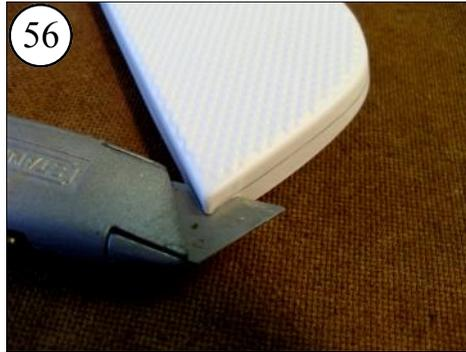
Sharp corners should be started with a razor using a rocking motion until the blade cuts into the plastic.
