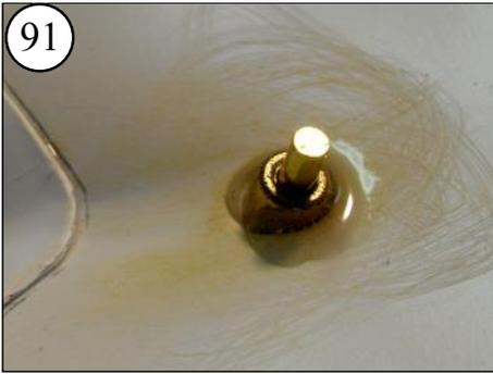
91 Just enough to encircle the bearing and fill the narrow gap between the bearing and the Hull Liner.
