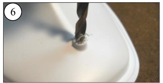
With a  $1/4^{\text{th}}$  drill bit, drill through the Rudder Bearing hole. Use gentle pressure. Let the drill slowly drill through the plastic to avoid it splitting.
