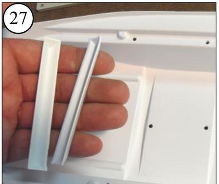
27 These are the Servo Tray Screw Reinforcing Strips. They provide a better anchor for the screw threads.
