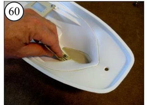
60 Sand all around the ballast and shaft area.
