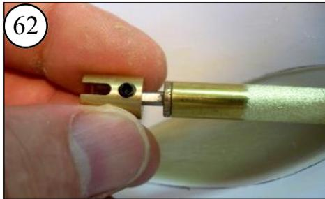
62 Insert the Stern Tube Assembly into the hull. Slide the 1/8 in Coupling End onto the shaft. Note the location of the flat on the shaft.
