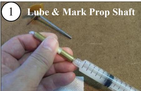
Squeeze the synthetic grease into the Stern Tube until it comes out the other end.
