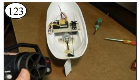
123 Turn the wheel of your transmitter to see if the rudder works. This is a LEFT turn of the wheel. If the rudder is opposite, then reverse the transmitter steering switch.
