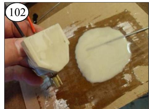
102 Put epoxy on the bottom of the Motor Mount.
