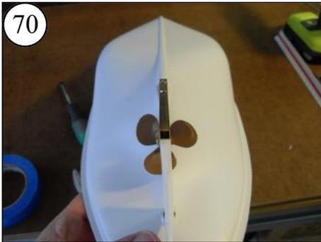
70 Align the Skeg with the Keel of the Hull.
