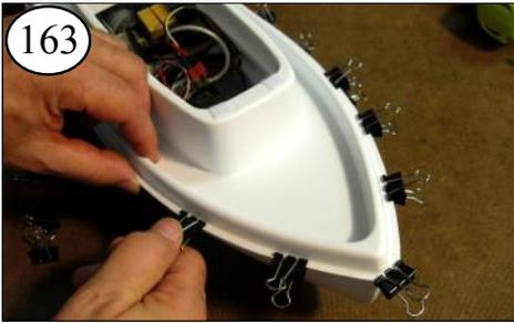
163 Align the bow-center and clamp. Then, work rearward left and right aligning the outside edges of the Hull and Deck flanges as you go.
