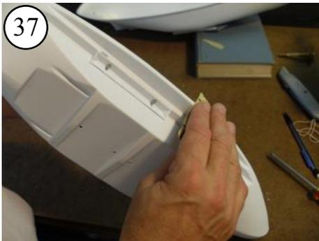
37 Don't forget the thin edges and bottoms of the floor ribs.
