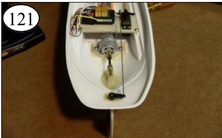
121 Align the rudder as shown. Now, tighten the screw on the E-Z Connector while holding the pushrod next to it. Any further adjustments can be made with the transmitter.
