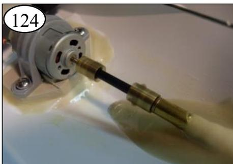
124 Pull the throttle trigger. The motor should turn the shaft freely.
