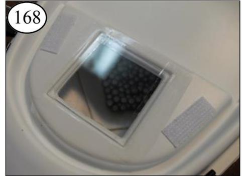
168 Tape the edges fully. This gives you access to the Rudder Arm and to the Prop Shaft Coupling.
