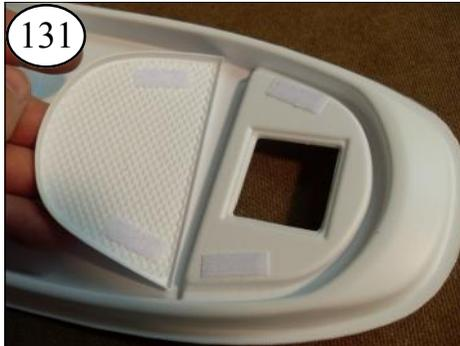
131 Remove the Hatch Cover and press the strips to set the adhesive.
