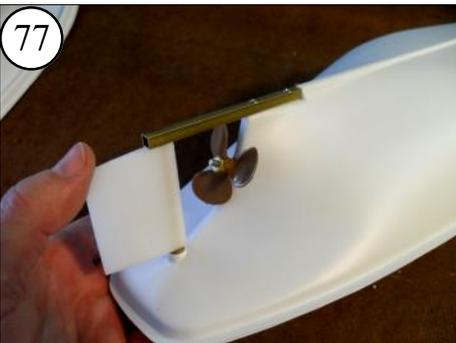
77 The Rudder should turn freely without binding.
