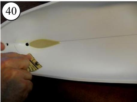
40 Sand the area inside the Hull below the marked line. Sand the areas around the rudder and prop shaft holes.
