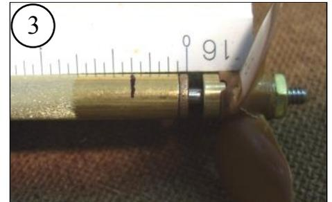
Put a mark on the Stern Tube about  $3/8^{\text{th}}$  of an inch from the end of the bearing.
