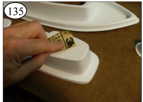
135 Sand the top of the Pilot House and underside of the Pilot House Roof. Glue together with CA.
