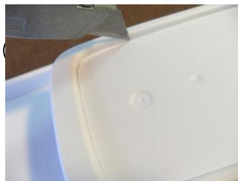
The Deck top recess is marked. Score 3-4 times and it will separate. Don't try to cut through the first time.
