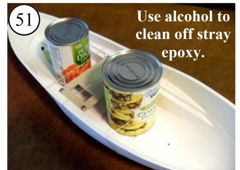
51 Use alcohol to clean off stray epoxy. A couple of cans or similar weights will help hold down the Liner until the epoxy has cured.
