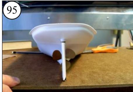
95 Check the shaft alignment. Confirm the motor is still centered and the mark on the side of the Prop Shaft is still aligned.
