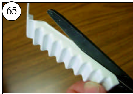
65 After rough-cutting, trim the sides of the stairs with scissors so they are flat. Trim the bottom step so its height
