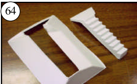
64 One set of stairs is marked for rough-cutting. Transfer the marks to the other 3 sets. One is a spare, in case you mess up one! Cut with a hobby knife. Flex to break apart.
