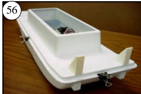
56 Temporarily clamp the Deck to the Hull to check the alignment of the Tow Knees.
