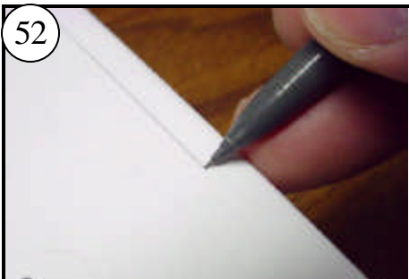
52 Using your finger as a guide, mark a line around the top of the Cabin about 5/16" from the edge.
