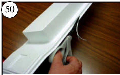
50 Trim the side of the Deck. Like the Hull, it may be easier to trim the sides holding the scissors upside down.
