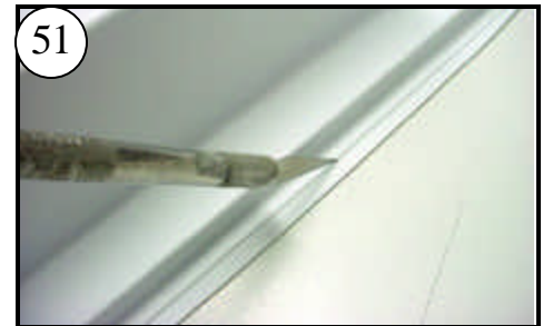
51 The Deck can be trimmed with a Hobby Knife by scoring the plastic along the trim line 3-4 times until the plastic separates.
