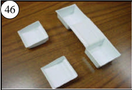
46 Trim the the Ballast Trays. These hold the Ballast Weights and allow easy adjustment of the waterline.
