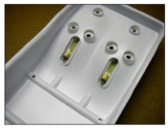
Make sure the excess doesn't cover the bearing on the front end of the stern tube. Use toothpick to remove excess glue.
