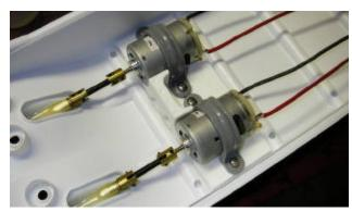
Sand the underside of the motor mount and the hull under it. Glue with filled epoxy. Slide the mount to align the dogbones. Leave some forward/rear play for the dogbones. Align 4 flankers with the 2 white foam blocks, then glue the bearings. Then, align & glue the rudders.
