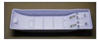
The liner is the same, but with two sets of openings for the 2nd drive & rudders. When gluing the liner, use a block or book under the rear shelf of the hull to ensure the stern is level with the table. Otherwise, you could end up with a slight twist in the stern, reinforced by the glued-in liner.
