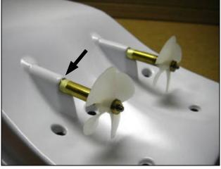
Mark each stern tube 1 inch from the rear Not much epoxy is needed under the shaft. end of the thrust bearing. Install with filled epoxy so that mark is just visible at the end of the stern tube opening.
