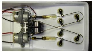
Scuff and use a drop of epoxy or servo tape to connect the servos together. Once cured, use 4 servo screws to attach the servos to the motor/servo mount exactly as shown. The rudders & flankers are strait fore & aft in this photo. The servo's arm and its three rudder-flanker arms must be parallel. See "rudder alignment notes".
