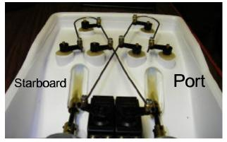
Note the port rudder arms are upright. The Starboard arms are upside-down. This separates the pushrods so they don't touch where they cross. Put a slight up-bend in each arm near the servo to align.
