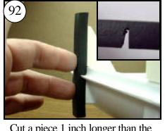
Cut a piece 1 inch longer than the height of the Push Knee. Notch it for the flange as shown in the inset photo. If you cut wrong, enough is included for 4 pads!
