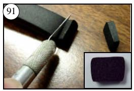
Pads for the Push Knees are cut by pressing a hobby knife or razor strait down through it. One side is slightly wider than the other. (Top of inset photo)
