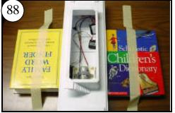
Push the sides of the Hull in a little as they stick out relative to the Deck. This will prevent the CA from bonding them
