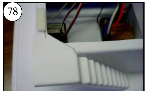
When installing Velcro to attach the 2nd deck, place it next to the stairs, not on top of them.
