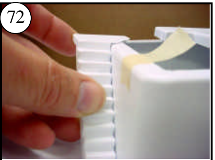
Rolling the top flange inward will level the upper steps. Too much and they could slant to the right.
