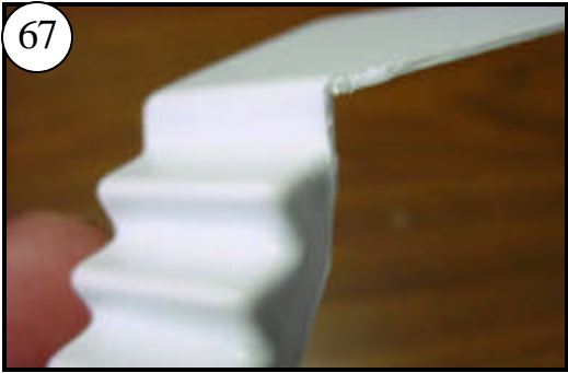
Trim this inside top corner to be flat so it will mount flush against the side of the Cabin. This top step will serve as a guide to align the 2nd Deck onto the Deck.
