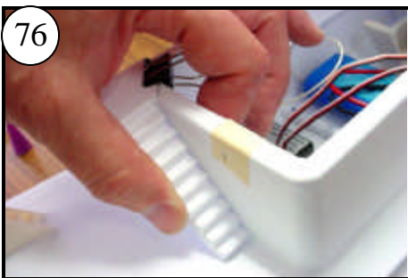
Align the top onto the Deck and clamp. Swing the Stairs against the Cabin and down onto the Deck. Hold in place 1 minute.
