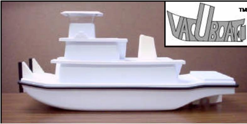
**Length: 21.5 in. Beam: 6.5 in. Draft: 2 in. Displacement: 6 lbs.**
