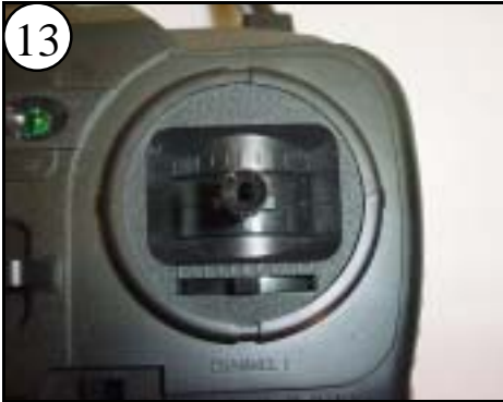
13 Center the Steering Stick in your 2-stick Transmitter. Center the Steering Trim below the stick as well.
