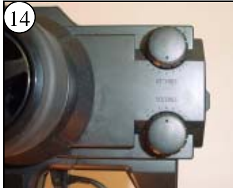
14 If you are using a pistol radio, center its steering trim as shown.
