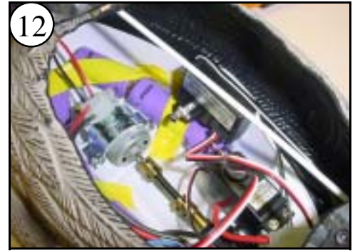
12 The mast will flex. Insert the end into the duck's neck. The other end (where the wire entered the mast) goes in the tail.
