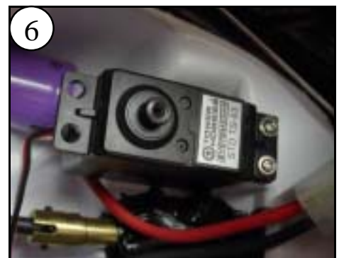
3 Use electrical tape to secure it. To prevent electrical shorts, cover all of the exposed connections. (Do a better job than this!)
