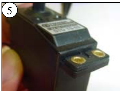
6 Install the Standard Servo into the two pre-drilled holes to the right of the Prop Shaft.
