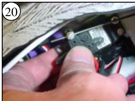
20 With your finger under the Servo flange, use your thumb to press the Servo Arm onto the Servo. Do not tighten the EZ-Connector yet.
