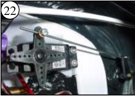
22 The EZ-Connector is ready to be tightened. The Rudder Arm and the Servo Arm should be roughly parallel as shown.
