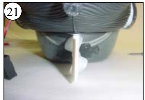
21 Align the Rudder to a straight-ahead position as shown.
