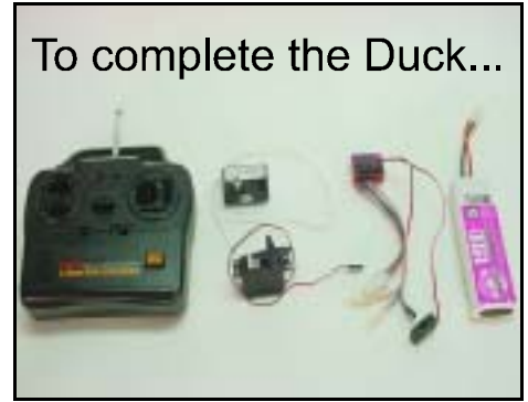
You will need a 2-Channel Radio w/ Std. Servo, an Electronic Speed Control (ESC), a 6 cell, 7.2 volt battery + charger.
