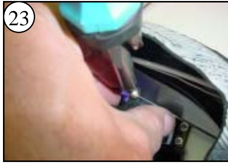
23 With your fingers holding the Rudder Pushrod, tighten the EZ-Connector with a small flat screwdriver.
