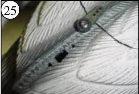
25 You can mount the on/off switch inside with Velcro® or cut mounting holes as shown and mount it outside.
