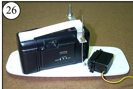
26 The servo arm should not strike the Deck when taking a photo. Adjust the Keeper so the servo travels just enough to click the shutter.
