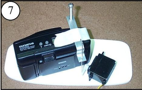
7 Orient the Servo to a position that allows it to pull the Pushrod straight down.
