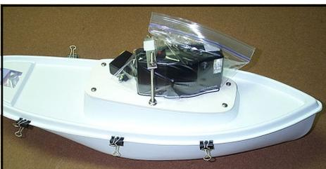
Put the camera into a zipper bag. Temporarily clamp the Deck to the Hull with 6 clamps.
