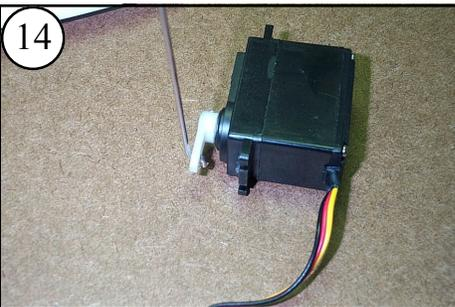
14 Attach the Z-bend end of the Shutter Pushrod to the servo as shown. Use the middle hole for a stronger pull.
