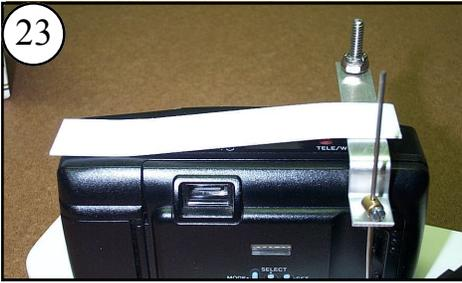
23 Lay the Brace on the camera. Trim one end if it overhangs the camera or the Shutter Arm.
