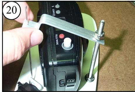
20 Center the Arm over the button. Press & hold for 15 seconds to bond the Button to the Arm.
