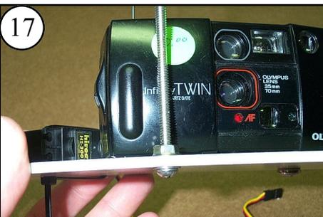
17 Attach the Shutter Arm Mounting Bolt as shown. The washer is under the Deck. The Shutter Mounting Bolt Flange Nut is on top.
