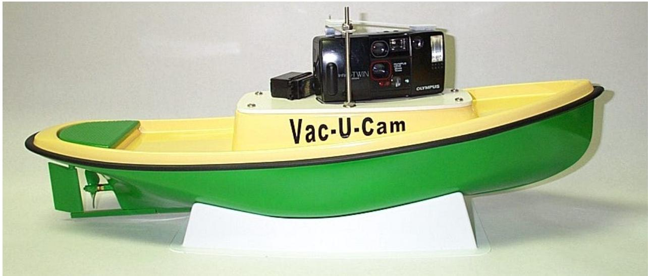
**Length: 22.5 in. Beam: 7 in. Draft: 2-3/8 in. Displacement: 4 lb.**
