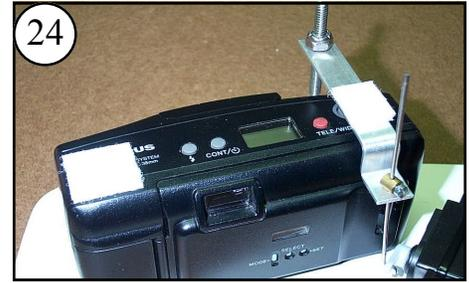
24 Attach Velcro to the camera and to the top of the Shutter Arm.
