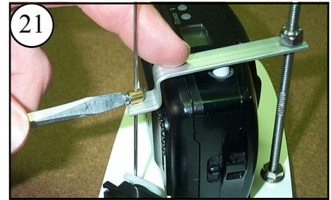
21 With the servo in the "take photo" position, push down on the Arm until the camera's shutter clicks. Tighten the Pushrod Keeper.
