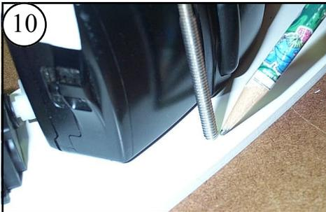
10 This camera has a sliding lens cover. I had to allow space for it to slide behind the Bolt.
