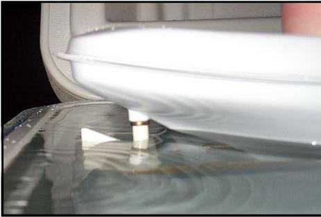
The stern waterline is 1/8th inch below the top of the fin of the rudder as shown.
