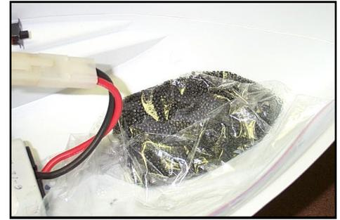
Combine the bow cup and bag ballast, mix with epoxy (in the bag), and press into the bow as shown.
