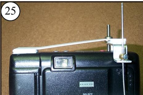
25 Place the Shutter Arm Brace as shown. This will keep the Shutter Arm centered in place.
