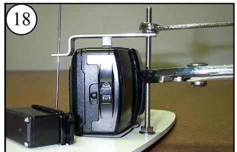
18 Grasp the Shutter Arm Mtg. Bolt with pliers at the center flat of the bolt. Tighten the Adjusting Nut with a 3/8 inch or 10 mm wrench until the Shutter Arm is level as shown.
