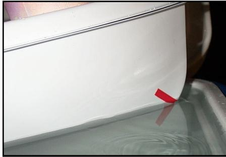
The bow waterline mark is in the center of the curve of the bow as shown by the red piece of tape.
