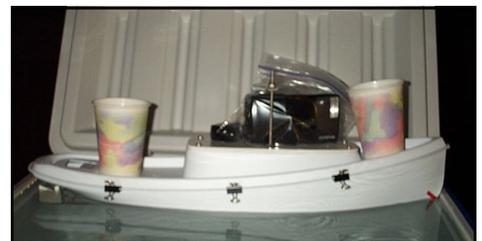
Set in water. Put two cups on deck as shown. Add weight to cups until you meet the waterline marks.
