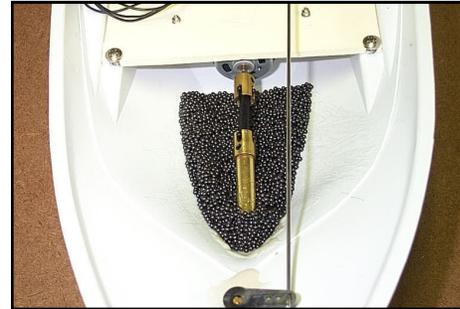
The stern ballast looks like this installed. Keep it away from the Motor-Shaft Coupling.
