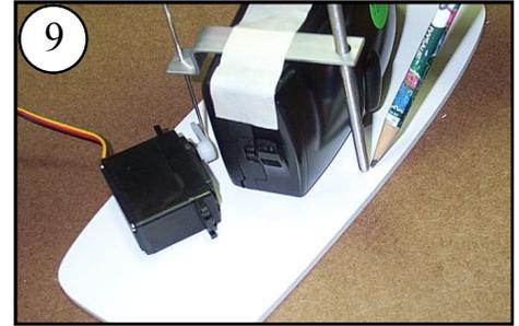
9 Drop the Shutter Arm Mounting Bolt straight through the Shutter Arm and mark the deck.
