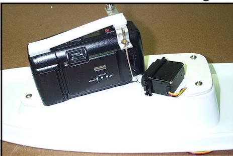
Attach the Camera Deck to the Cabin with 4 screws. Tighten gently until snug.
