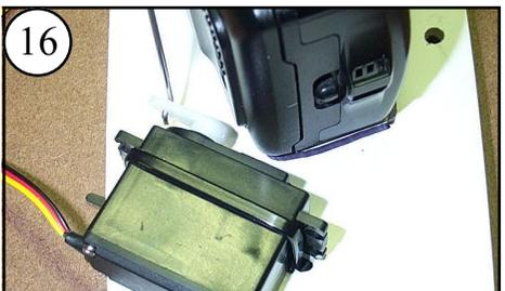
16 The attached servo will look like this from the top. The servo is in its "take photo" position. Set this by connecting the servo to the receiver & battery. Throw the transmitter stick to "take photo" position. Turn off the receiver.
