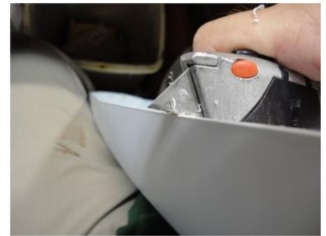
Smooth any high spots. Use the sandpaper or lightly scrape with a knife. The sealant used in attaching the deck will bridge any low spots so it does not have to be perfect. Note the Transom has a curved top to match the crown of the deck.
