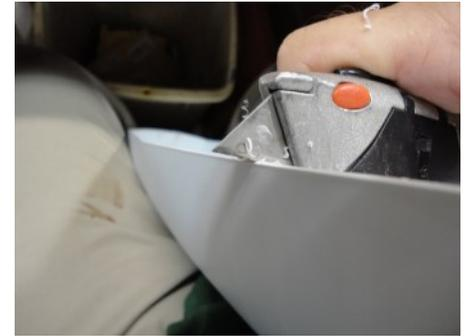
Smooth any high spots. Use the sandpaper or lightly scrape with a knife. The sealant used in attaching the deck will bridge any low spots so it does not have to be perfect. Note the Transom has a curved top to match the crown of the deck.
