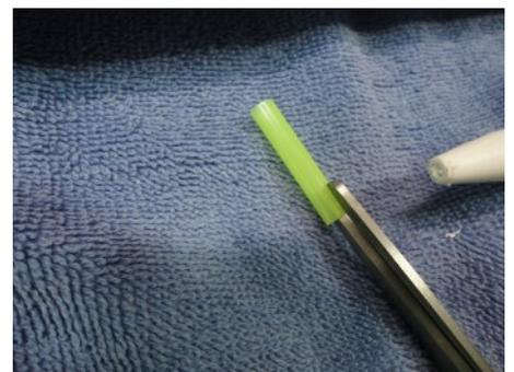
The nozzle of the tube of sealant is too large for the Deck groove. You need to extend the nozzle with a thin flexible tube. A plastic drinking straw works well. Clip off about an inch. Cut two short slots on one end.
