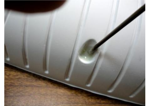
Fold-in an equal volume of filler powder & mix well. Scoop up some and distribute around the inside of the chosen anchor point. The insert is form-fit so little epoxy is needed.
