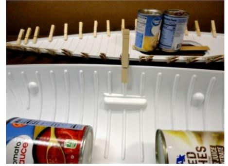
The cans will hold down the Hull Liner. You start clamping the top at the center. Lightly pinch the sides together with your left hand while you clamp with your right. Center the clothespin on the rib.
