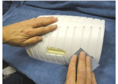
Sand inside the Hull at the transom back and sides. Carefully support the back of the transom while sanding as it is very thin. Sand the outside of the Transom Reinforcement. If the reinforcement epoxy is cured, sand the Hull Liner as shown. The folded towel will allow you to support the shape while sanding.
