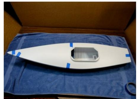
Working from the stern to the bow, tuck the Hull into the groove of the Deck. Add tape at the middle when you are farther along. When you finish at the tip of the bow, add a piece of tape there. Press evenly to ensure the deck is fully engaged onto the hull. Adjust the tape to remove any slack. No need to tightly pull the tape. It is just there to hold things in place.
