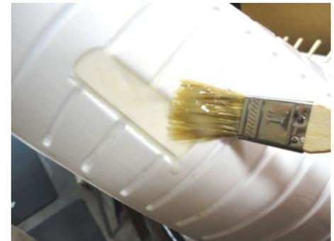
Mix 1-Pump of West Systems Epoxy and add 1 level tablespoon of filler. Brush onto the Hull Liner like you did the Deck Liner. When you are done, a little extra around the crossmember inserts will help strengthen this area. **Don't use all of the epoxy. Save some for the Transom Reinforcement.**
