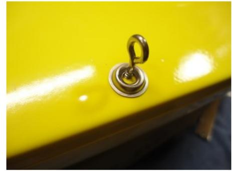
The stainless steel flanged finish washers help support the screw eyes from side loads. Start the screw eyes by hand.
