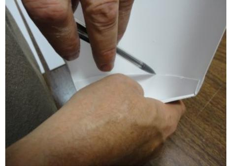
Carefully trim off the marked top of the Transom Reinforcement by scoring with a knife or use scissors. If scoring, lightly score once then repeat until you can break off the scrap. Set the Transom Reinforcement back into the transom firmly seated in place and mark the edges in the Hull for sanding.
