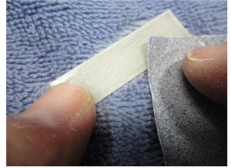
Sand the underside of the King Post Upper Mount. Sand inside the Transom inside the raised rectangle where the Transom Backer will be glued. Sand one side of the shorter fiberglass backer. Sand both sides of the white plastic spacer and the backer for the Mast Step. The short backer is for the Transom.
