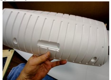
In the Hull Liner you will need to glue inserts into the two shelves that support the Crossmember and the two marked Anchor Points. Sand the 4 reinforcements and separate them from each-other. Each crossmember reinforcement is different. 8
