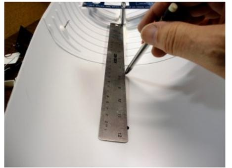
Drill into the two reinforced Anchor Bump from the side, direction of the pull, as to not pierce the Hull. Screw the Screw Eye into the bump just as far as the threads. Install the Rudder & Rudder Servo Mount: Using a straight edge, mark a light pencil line about 4 inches from the Rudder Mount hole toward the end of the Keel Shoe.
