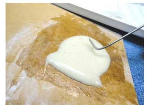
Sand the back of the ledge as well. Sand the **underside** of the Cockpit Cover in the same area. Mix two 1-inch circles of epoxy and add the same volume of filler. Put a 1/4-inch bend on the end of a paperclip to distribute the filled epoxy.
