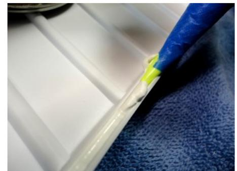
Don't try to do this in a continuous movement. A "stitching" move where you stop, letting the sealant build up then back up a fraction of an inch and let it fill again works well. High spots will happen. They can be scraped out later before you bond the Deck to the Hull. No hurry, take as long as you need. If sealant starts oozing out of a hole in the tape you may need to tape over or make a new nozzle and start again.
