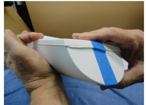
Move along seating the Deck over the Hull. As you seat the Deck, re-position the tape. No need to pull hard. The sealant will stay in place. The tape just holds it there. There will be lots of oozing at the Transom. Once the Deck is on the line, add tape to the sides of the stern of the boat.
