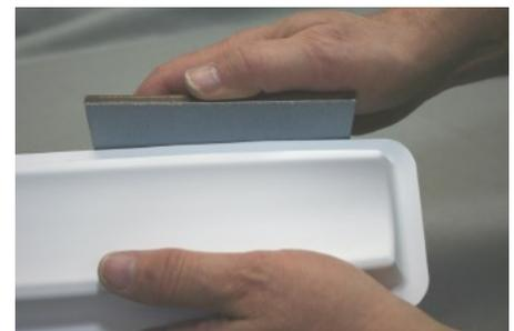
Bending down at the score will break the plastic along the scored line. Then, bend up to separate it cleanly. Don't tear or it will leave an uneven edge. You can cut with scissors if you prefer. Either way, any rough edges can be smoothed out with the included 100 grit sandpaper.
