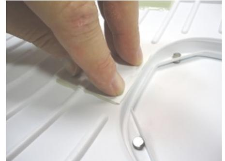
Attach the Mast Step Backer then apply filled epoxy to the King Post Upper Mount and set into place.
