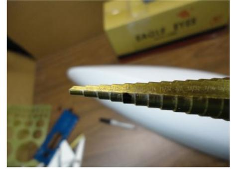
These are the Hull drill locator dimples. You used them earlier to center the Hull Liner into the Hull from the inside. **Practice drilling through a scrap of this plastic with a step drill.** Use a slow speed setting. Be patient. Use little pressure. Note the drill diameter markings on the step drill. Locate the 1/4-inch mark for the Keel holes. Step drills are recommended because they are better than standard drills at remaining centered as they drill into the plastic dimple.
