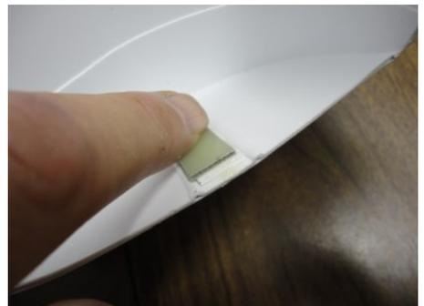
Add filled epoxy to the white plastic spacer. Press the shorter fiberglass Backer into the spacer, the end aligned to the bottom end of the spacer. **Important:** This leaves the top of the fiberglass backer about 3/8-inch down from the top of the transom. This is to allow room for the Transom to fit into the Deck groove later.
