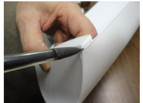
Set the Transom Reinforcement into the Transom end of the Hull and align to the sides of the hull. Mark along the Transom top and Hull Sides for trimming. Be careful not to move or shift the reinforcement while marking.
