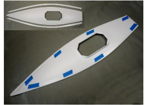
**Lightly score around the inside of the cockpit opening from the top of the deck.** Repeat until the center pushes out. **Score the deck reinforcing liner from its underside.** This leaves a raised lip around the top of the liner's opening. Set the scraps aside for testing paint or practice drilling holes. Tape the temporary deck clamping strips on top of the deck, even with the deck's edges.
