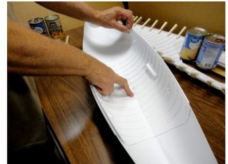
You can tape them in place. **Practice** setting the Hull Reinforcing Liner into the hull without touching the sides to prevent epoxy from rubbing off onto the hull. Repeat centering on the two locator bumps with your fingers and confirm the location with the end-marks you drew on the hull. The Hull should be sitting directly on the work table. To keep it from falling over, steady the sides with a folded towel or other object that won't get in the way of clamping.
