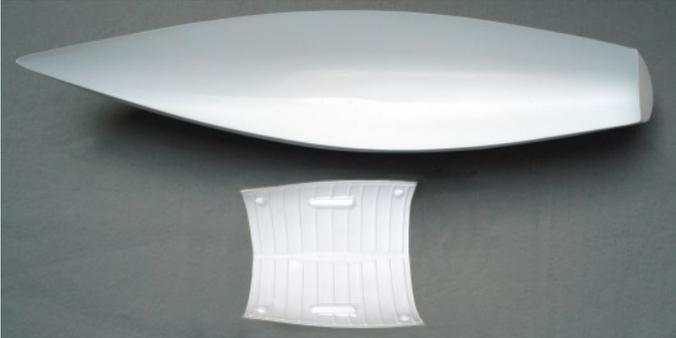
**Hull with integral Transom, Hull
