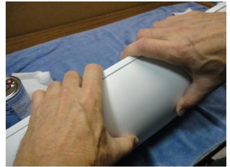
Tape the bow. The Hull should be in the groove of the Deck, but not fully seated. Using light pressure, push the Deck onto the Hull until you are at the indicator line you drew earlier.
