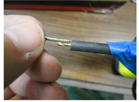
A bent wire will help remove any excess sealant. The sealant is messy stuff so you may want to leave the excess sealant alone for a better appearance. If you are using Anchor Points in the Hull, they need to be drilled and installed now. Otherwise, skip this step. Repeat the Drill Depth Gauge setting. This time with a 1/16-inch (1.5mm) drill bit the length of the eyelet threads. Secure the hose with tape or it will slide off of the smaller drill.
