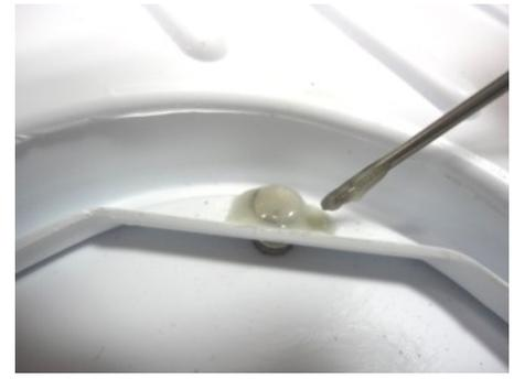
Confirm the 3/8-inch space and clamp with a clothespin. Put some filled epoxy over and around the 4 Cockpit Magnets to better hold them in place. If your epoxy is beginning to harden, mix a small fresh batch to do this. Set aside to cure.
