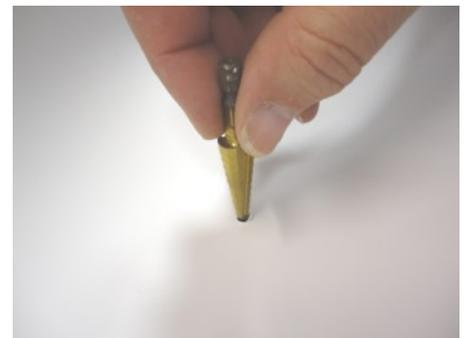
Clean off old Sharpie markings with alcohol. Locate the 3/16-inch point on the drill and mark that section plainly with the Sharpie marker. Drill the Rudder hole to a 3/16-inch diameter. By hand, you can use the step drill to de-burr the hole on the inside.
