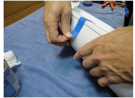
Like earlier, engage the angled transom first, securing the Transom end with a piece of tape. Don't try to reach the line on the Transom with the Deck yet. Work toward the bow, tucking in the hull. At the middle, add tape to secure.
