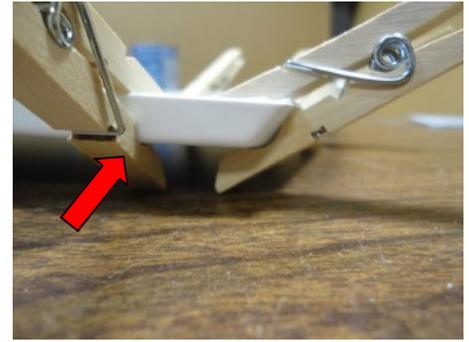
Clamp 3 more clothespins keeping the Deck Reinforcing Liner centered to the deck. Clamp two more at the end of the stern. There are no ribs there but still keep the deck corner into the notch of the clothespin.
