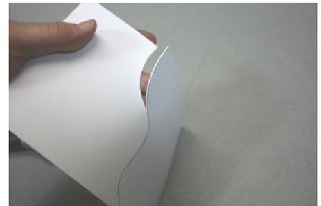
Styrene can be cut by scoring and breaking, or with scissors. The first score should be very light while concentrating on accuracy. The second and third score is made with more pressure and will follow the first. Repeat scoring the line until the part separates or after 2 or 3 scores, bend the plastic to break it.
