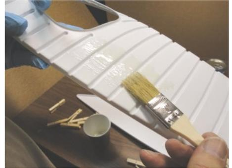
Mix 1-Pump of West Systems Epoxy and stir in 1 level tablespoon of filler. Brush the filled epoxy on to the Deck Liner. Hold the brush almost flat against the surface and very lightly brush the surface. Flat strokes will distribute the epoxy on the surface without it getting in to the grooves. If it gets into the grooves, scoop it out with the brush.
