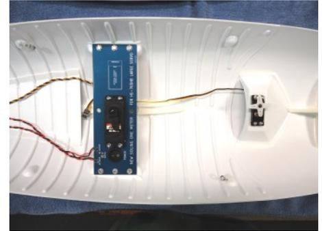
Run the double folded sandpaper back and forth in the grooves of the Deck. **Remove it often** to clean off any plastic debris. Check it for loss of granules and refold as needed to finish the job. Now is a good time to install any equipment you plan to use in the boat. Velcro® for the Battery Tray, wiring and Servo for the Crossmember and the Rudder Servo. Tape down any loose wires to keep them away from the Deck to Hull joint. No need to install the rudder or linkage at this time.
