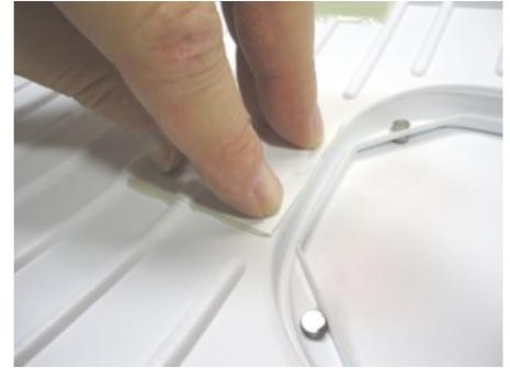
Attach the Mast Step Backer then apply filled epoxy to the King Post Upper Mount and set into place.
