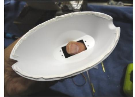
Drill a 1/8-inch hole at each corner of your measurements and connect the holes by scoring through with a knife. Use the rudder servo to locate and drill its mounting holes with a 1/16" drill bit. Apply a thin bead of sealant and set the Rudder Servo Mount into the hull aligning it with the Rudder Mount and the pencil marks you made earlier.
