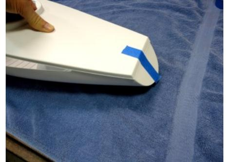
Because the Transom is angled, you have to engage the Deck into the Transom first, at an angle. Once the Deck is in on the Transom, put a piece of masking tape over the end to hold it in place.
