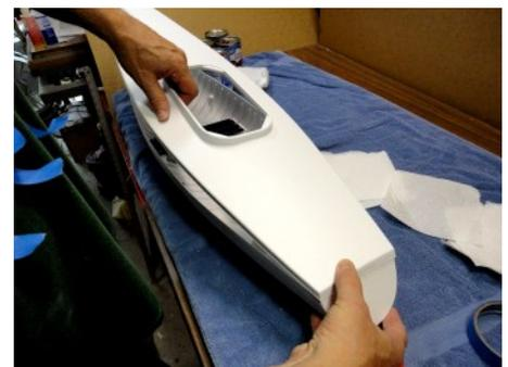
This bead of sealant will work. It is continuous with no gaps. It is just below the height of the Liner's side of the groove and about halfway up the edge of the Deck. In preparation to attach the Deck to the Hull, have 5 or 6 pre-cut pieces of tape nearby. Remember to tape down any loose wires in the deck. As before, engage the Transom first while holding up the other end of the Deck.
