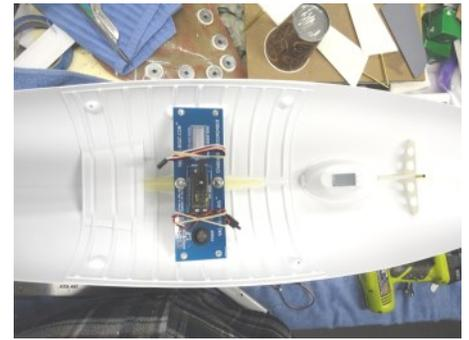
Apply a thin bead of sealant to the side flanges of the Battery Tray and press into the hull. Wipe away any excess sealant.
