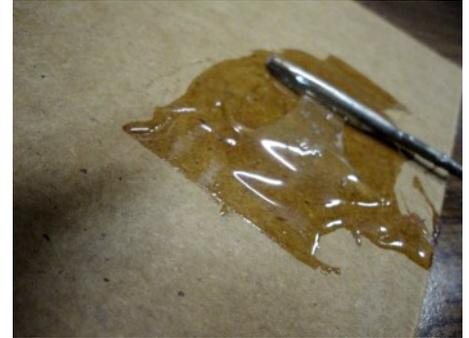
Lay out the shelf inserts and anchor point inserts near where they go to avoid mistakes. Pour two 1-1/4-inch circles of 30 minute epoxy and mix. A steel rod works well for this. A 1/8" diameter rod was used for these photos.
