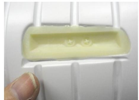
Press the insert into the epoxied recess. Wipe away any excess epoxy. Repeat for the other anchor point and the two Crossmember shelf inserts.
