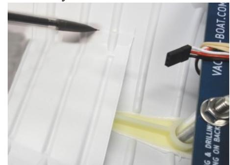
Press into place. Wipe away any excess sealant. Set the pre-trimmed Battery Tray into the Bow. It only fits into this location. Trace its outline onto the hull with a pencil. Sand the Tray and Hull at the point of contact. If you plan to put a strip of Velcro® on the battery tray, do it now, before you apply sealant or do it tomorrow after the sealant has cured some and before you install the Deck.
