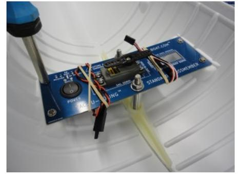
Now is a good time to mark and drill the servo screw holes into the crossmember. Use a 5/64" (2mm) drill for this kit's servo screws. **READ THE WARNINGS** on the crossmember when drilling holes or enlarging openings. Secure any loose wires on the Crossmember. **TEMPORARILY** install the crossmember with mounting screws. **ADVANCED:** Now is a good time to check the alignment of the keel to the rudder shaft if you want to do this.
