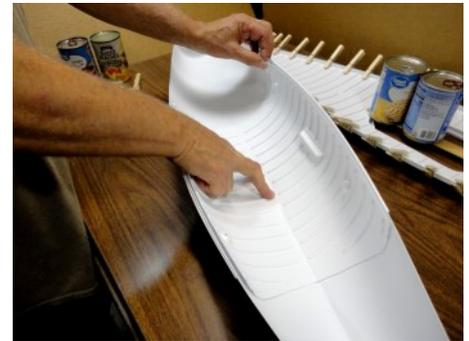
You can tape them in place. **Practice** setting the Hull Reinforcing Liner into the hull without touching the sides to prevent epoxy from rubbing off onto the hull. Repeat centering on the two locator bumps with your fingers and confirm the location with the end-marks you drew on the hull. The Hull should be sitting directly on the work table. To keep it from falling over, steady the sides with a folded towel or other object that won't get in the way of clamping.
