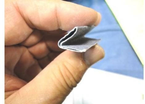
Firmly pinch the piece of Sandpaper over the top edge of the Hull and slide back and forth to roughen the surface. Open the piece and remove plastic debris often. The horizontal scratches will help the sealant grip the plastic. Sand half of the hull then refold the piece to sand the other half. Cut another piece about 1-1/2-inch square. Fold in half then fold again. Press tight.
