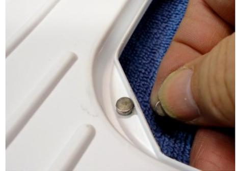
The Hull is ready for the Deck. Leave the Hull on the Keel to cure overnight, approximately 24 hours and seal the end of the caulking tube to keep fresh until then. **Two more things to do to the Deck before tomorrow.** The magnets you glued to the underside of the Deck were sanded-side-down into the epoxy. You clamped that magnet in place by putting another magnet under it.
