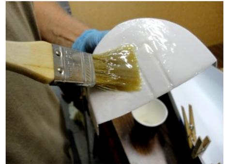
You will notice that in between the clothespins there may be gaps between the Hull and the Hull Liner. Clamp these gaps with another clothespin, not clamping the rib this time. Look for any epoxy oozing out of the top and clean it while it is still uncured. Apply the filled epoxy to the Transom Reinforcement.
