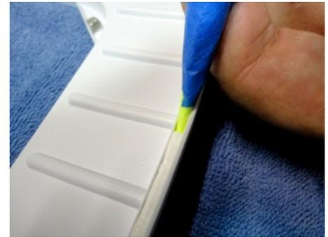
Adding weights to the deck will help hold it in place on the towel. You will need both hands to apply the sealant. Insert the straw-nozzle fully into the groove. As you dispense sealant, **let it fill the groove from the bottom-up** until it is just below the height of the Deck Liner's edge as you pull the nozzle along.
