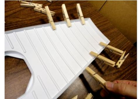
Center the tip of the Deck Liner to the tip of the Deck. Clamp 4 clothespins to the 2nd & 3rd ribs as shown. Check that the cockpit opening is still centered. Starting at the stern end, alternating left then right, attach clothespins to every other rib working toward the cockpit.
