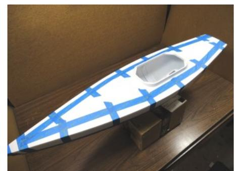
Keep working around the boat until everything is aligned. No additional tape is necessary. Before sealing up your tube of polyurethane sealant, run out several 3/16-inch diameter beads of sealant 6 to 8 inches long onto a plastic bag and mark the date on the bag. Store the beads of caulk with the Hull as it cures. To test the strength of the cured sealant, remove one of the beads and pull & stretch it to get an idea of how much the sealant on the hull has cured at that time.
