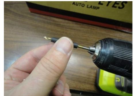
Remove the Crossmember. These holes will be drilled with a 3/32-inch drill. Insert the drill bit into your drill and slip the rubber hose depth gauge over it.
