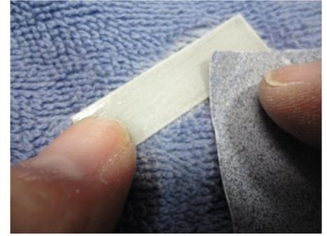
Sand the underside of the King Post Upper Mount. Sand inside the Transom inside the raised rectangle where the Transom Backer will be glued. Sand one side of the shorter fiberglass backer. Sand both sides of the white plastic spacer and the backer for the Mast Step. The short backer is for the Transom.
