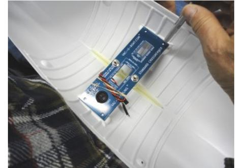
Set the Crossmember onto the Keel Bolts. While holding the Crossmember to prevent rotation, install the two 1/4-inch stainless steel washers and the two 1/4-inch Keel Nuts. Just snug with wrench. Do not over-tighten. While squeezing the hull between your hand and stomach, check that the ends of the crossmember are square to the ridge on the back of the shelves then mark the 4 screw holes onto the shelves.
