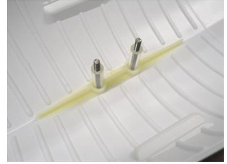
Set the Keel Shoe into the hull centered on the keel holes and mark the shoe's outline. Sand the underside of the shoe and sand the shoe's outline in the hull. Set the hull onto the Keel. Place the Keel Mount Tubes over the Keel Bolts with the end that is grooved on the bottom (arrow). Set the Keel Mount Shoe over the two tubes.
