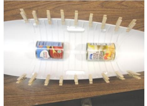
Notice how the clothespin is clamping the end of the rib and the top edge of the Hull Liner. The Spring is not touching the plastic. Continue pinching and clamping every other rib until both sides are done.
