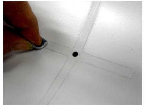
Insert the Rudder Mount into the hole with the **pointed end toward the Crossmember**. Align the point to the middle of the pencil line. Remove the Rudder Mount and sand the marked area. Also sand the corresponding bottom of the Rudder Mount.
