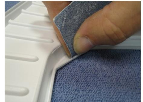
**Hazard:** Rare earth magnets are plated with Tin, Chromium, Cadmium or other harmful metals. Avoid dust and debris from scuffing them. Sand them outside. Take the row of magnets and sand one end to roughen the surface. Take a magnet from the other end and snap it over the sanded magnet. Repeat until **one side** of each magnet is scuffed. Sand the **underside** of each corner shelf of the Cockpit Opening.
