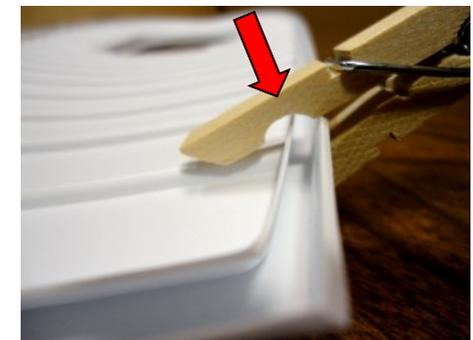
Take a clothespin and clamp the rib of the Deck Liner to the Deck near the Transom. Adjust it until the corner of the deck clamping strip falls into the notch of the clothespin. The flange of the Deck Liner is within the other notch in the clothespin. **5**
