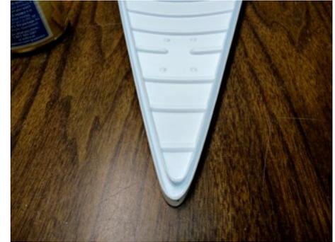
Remove the towel. Set the Deck upside-down onto the work surface. Set the Deck Reinforcing Liner into the Deck using the cockpit opening to align the Liner to the Deck. You will notice an even spacing around the perimeter. This will be the groove of the tongue-in-groove seam for the hull.
