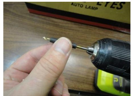
Remove the Crossmember. These holes will be drilled with a 3/32-inch drill. Insert the drill bit into your drill and slip the rubber hose depth gauge over it.
