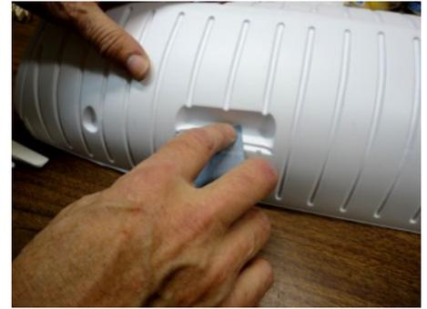
This is the correct Crossmember shelf insert for this side. It fits flush and evenly into the opening. The anchor points inserts fit any anchor point. Sand the insides of the two shelves and two inserts you marked.
