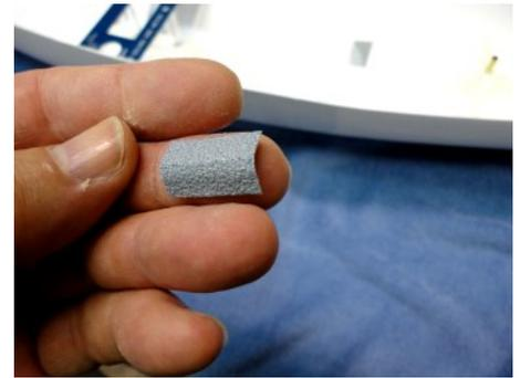
Carefully tape along the line on the Transom. Sealant will ooze out of this end. The tape will help with the clean-up. Cut a piece of the double-sided Sandpaper roughly 5/8-inch x 1-inch and fold it in half long-ways as shown.
