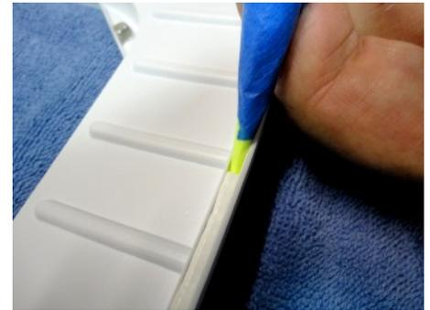
Adding weights to the deck will help hold it in place on the towel. You will need both hands to apply the sealant. Insert the straw-nozzle fully into the groove. As you dispense sealant, **let it fill the groove from the bottom-up** until it is just below the height of the Deck Liner's edge as you pull the nozzle along.
