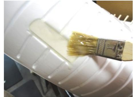
Mix 1-Pump of West Systems Epoxy and add 1 level tablespoon of filler. Brush onto the Hull Liner like you did the Deck Liner. When you are done, a little extra around the crossmember inserts will help strengthen this area. **Don't use all of the epoxy. Save some for the Transom Reinforcement.**
