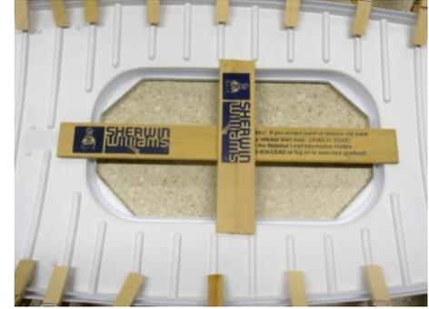
At the bow-end of the deck, put clothes pins on the two ribs shown next to each other. Then continue every other rib to the bow as shown. Put a single clothes pin at the tip of the bow. Set your paint stirring sticks into the cockpit. Long stick first with the left end (bow end) covering the five locator bumps next to the cockpit opening as shown. Put the short stick on top.
