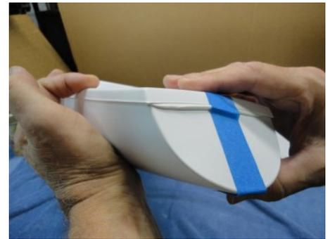
Move along seating the Deck over the Hull. As you seat the Deck, re-position the tape. No need to pull hard. The sealant will stay in place. The tape just holds it there. There will be lots of oozing at the Transom. Once the Deck is on the line, add tape to the sides of the stern of the boat.
