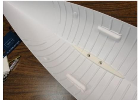
Use a Sharpie marker to plainly mark the 1/4-inch part of the drill. Drill the two dimples to 1/4-inch diameter. Turn the Hull over and set the Keel Mount Shoe into the hull.
