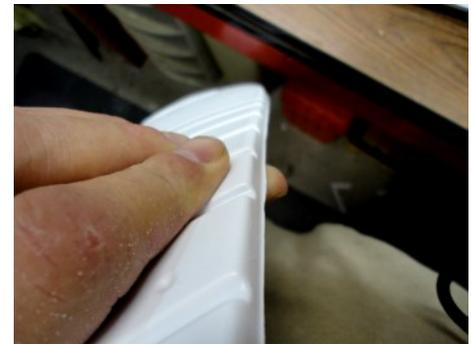
Lay out a towel & turn over the deck onto the towel. Sand the **UNDERSIDE** of the Deck thoroughly. Use a crisscross or circular pattern to roughen the surface for the epoxy to bond well. Sand the **TOP** of the Deck Reinforcing Liner. Check the edge trim of the Deck Liner. Use the sandpaper to straighten any uneven spots like at my thumb.
