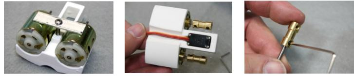
Install the motor clamp and screw. Tighten only until snug. Install the servo with the wire running toward the stern of the ship as shown. Drill 1/16" holes at the dimples in the mount and attach with the two screws included with the servo. Insert shafts fully into motor coupling & lightly tighten one set screw.
