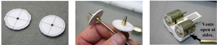
Prop templates can help you align the prop shafts to the hull and rudders in a scratch-built drive system. Glue to flat plastic scrap. Drill 1/8 hole at center & sand to the outer ring. Mount at the center of the threaded part of the shafts temporarily while gluing the motors and stern tubes in place. The inner ring is the prop's 1-inch diameter. The space between the rings is the clearance you want between the prop and the hull.
