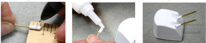
Mark the tube 1/8" from the end. Put a tiny amount of CA around the end of the tube and insert 1/8" into the gun.
