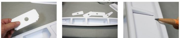
Save the scraps. Repeat for the other three deck openings. The side openings have three sides that are easy to mark. The bottom is located by using the side of a pencil to mark the change in the hull curve.
