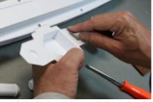
Optionally, you can add some foam inside the 2nd deck to help the boat sink upright in battle. Sand the raised portions of the top of the deck house. Sand the corresponding areas under the 2nd deck. **Important - Leave out any foam in the 2nd deck if installing a bow cannon as large holes would be drilled there.**
