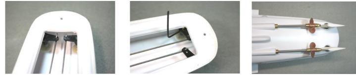
Insert the rudder shaft through the mount and rudder arm. Leave a little up and down play in the rudder to prevent binding. Tighten the rudder arm screws against the flats of the rudder shafts until snug. Turning the rudder will give you wrench access. With the servo centered, insert the rudder pushrods into the servo arm EZ-Connectors as shown.
