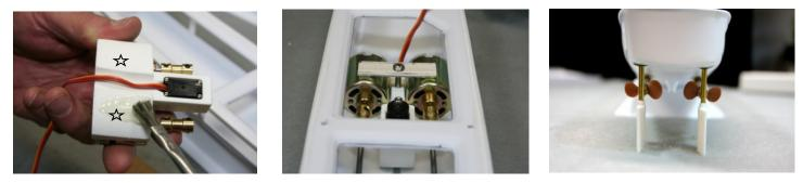
Brush filled epoxy on the underside of the motor mount. **No epoxy near the tunnel to avoid the servo wire.** Set the motor assembly into the hull at the marked location. Hold in place. Attach shafts aligning the flats with the coupling set screw holes. With the boat on the stand, insert the rudders into the rudder mounts for reference.
