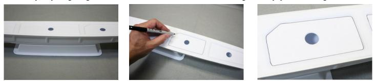
The stand fits the hull as shown. The right end of the stand lines up with the rear of the bilge keels on either side of the hull. Outline the bottom of the sub-deck openings with a pencil. Use slight outward pressure on the pencil so it will follow the outline of the recess. The mark helps you see where to score the opening. 4
