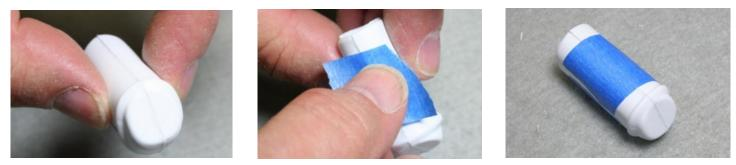
Fold together and align the seam. Hold for 15 - 20 seconds. Secure with tape and let it dry at least one hour.
