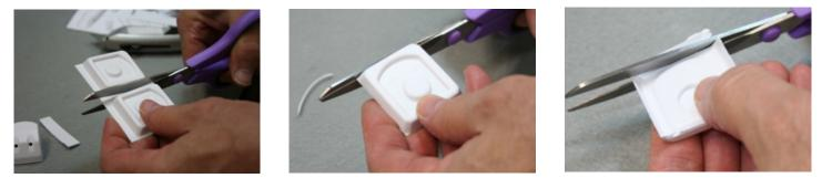
Separate the three gun bases. Trim away the edges as shown. Turn over and trim closer but don't cut the raised area.
