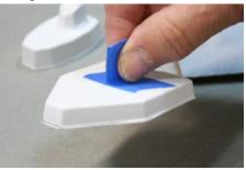
Like the gun housings, use the sanding block to sand away the edges left by the scissors. The thinner pieces are easier to hold with a handle made from masking tape.
