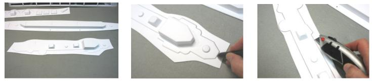
The 2nd deck sits on top of the deckhouse. It has a raised outline. Mark the bottom of the outline with a pencil and use your knife to lightly score the line. Repeat scoring 3-4 times until the edges will break away.
