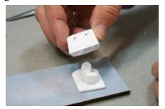
Gun housing and base ready to glue. Put superglue around the inside edge of the housing. Set the base on a flat surface that the glue won't damage. Don't forget the small piece of foam.
