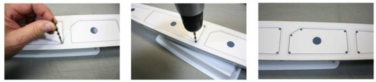
Use a 3/16" drill to round the corners by drilling next to the marked line at each corner. Do this for all 4 openings.
