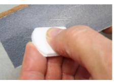
Trace around the raised area to guide your cutting. Cut to the line with scissors. Sand away any edges missed.
