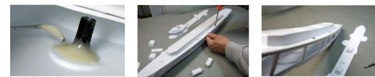
Inside the hull, add filled epoxy to reinforce the stems of the rudder mounts as shown. Use a bent wire to reach around to distribute the epoxy. Attach the deck to the hull with the center 4 screws. The deck and hull are curved. Gluing on the 2nd deck with the deck attached to the hull will help preserve the curve of the deck to match the hull's curve.
