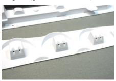
Consider the up-angle for your gun barrels. Mark each gun and drill with 1/8-inch drill, each at the same angle.
