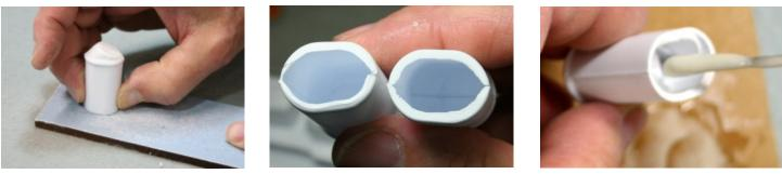
Holding at the base, with light pressure, sand the bottom flat to where the sides of the stack begin to curve inward. Take your time. Check frequently to make sure it sits straight on a flat surface. Before & After photo. Insert a piece of foam and put mixed epoxy inside the stack on the foam and along the inside of the glued seam to strengthen the stack and make it float. Set aside for the epoxy to cure. 13
