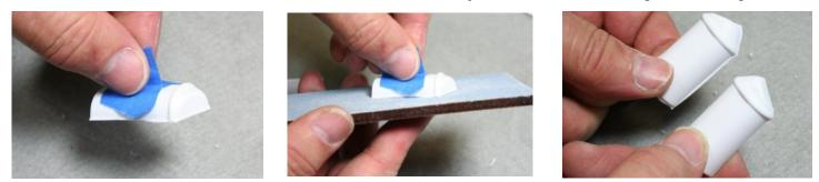
Easier to hold the stack half for sanding. Sand to a flat surface. Don't press too hard. Before & After sanding.
