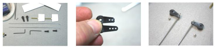
Get the two pushrods, rudder arms, set screws and hex wrenches. Cut away the outer hole of each rudder arm as shown and round the two corners a little. Install the Z-bend of each arm from underneath into the outer hole as shown. The set screws will install from the bow-end.
