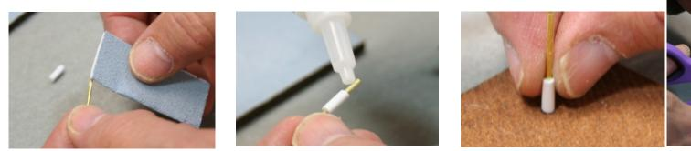
Sand 1/4 inch of the end of a brass rod. Slip the 3/8" piece of tube over that end. Add a little CA around the end of the rod and press the tube over the rod until even with the end of the brass rod to form a gun barrel. Make 6.
