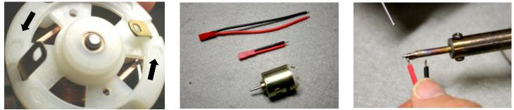
Now is a good time to solder a wiring harness to your motors while they are out of the hull. Next to each brass tab, there is an embossed + and - to indicate the positive pole and negative pole of the motor. Shorten the female JST connector to about 2-1/2 inches. Strip the insulation at the ends. "Tin" the wires by applying solder to them, 16 even if they are "Pre-tinned" silver.
