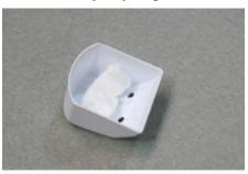
The sanded base has smooth turned-down edges. Sand the inside bottom of the gun housing. It is a good idea to put a piece of foam inside the housing for flotation in case your gun gets shot off of the deck.
