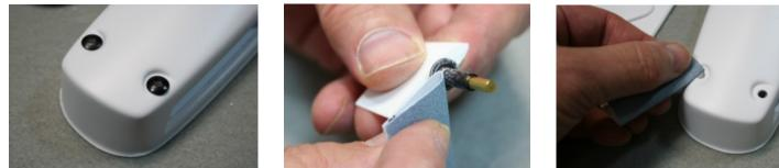
Remove the deck. Test fit the rudder mount. It should drop in and sit flush. If it binds, enlarge the hole a little with the 3/16 inch drill. Sand the underside and stem of the aluminum mount and the inside of the recess.
