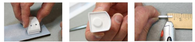
Press the gun housing over the base and hold for 10 seconds. When picked up, the bottom of the gun housing should look like this. Repeat for the other two guns. Cut a 3/8-inch long piece of plastic tube.
