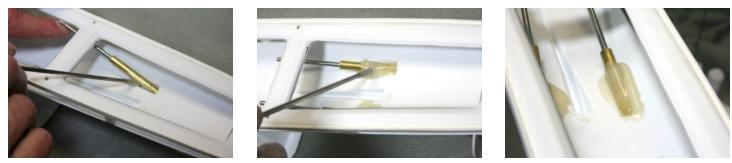
While holding up the inside shaft end, use a rod or narrow brush to force epoxy under the stern tube into the hull shaft journal. Rotate the tube to distribute the epoxy. Clean any grease off of your fingers to avoid contamination.
