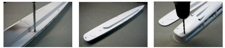
Insert the #6 x 3/8 inch Phillips pan head screws. Keep them straight as they thread into the sub-deck until just snug. Don't over tighten. Next time, start them by hand and lightly snug with screwdriver. Use a 3/16 inch drill to drill into the center of the rudder inset at the stern of the hull. Wallow out the hole a little so the rudder base will fit.
