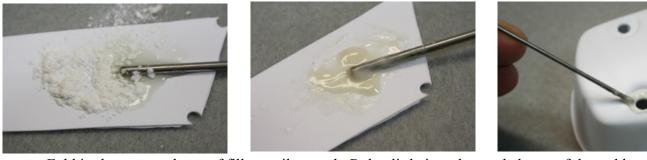
Fold in the same volume of filler until smooth. Rub a little into the sanded area of the rudder recess.
