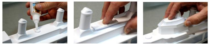
The torpedo launcher points toward the bow of the ship. The pilot house front edge lines up with the base under it. Note the raised walls of the bridge railing hang over the sides of the base under it.
