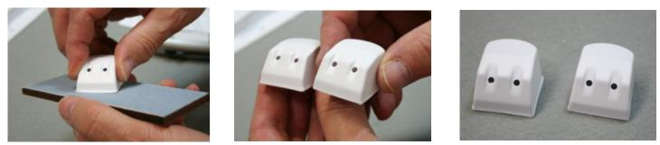
Sand the gun housing back and forth on the sanding block, rotating frequently to remove the curve evenly. Sand only until the curve is mostly gone. Before & After sanding.
