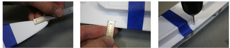
At the bow (front end) make a dot centered one-inch from the tip of the deck. On the sides, mark the dot 3/8 inch from the outer edge. Drill 3/32 holes through the deck & sub-deck at each dot. (Six holes.)\*\*
