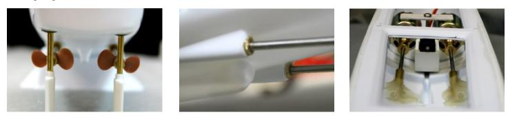
Visually center the two props to the rudders. The motor mount will slide a little left or right. Check the position of the stern tubes. Note the servo is approximately centered to the keel groove in the floor. Check the distance from the end of the prop shafts and the leading edge of the rudders. When everything is lined up, let the epoxy cure. Check as it cures to make sure nothing moved while the epoxy was still liquid.
