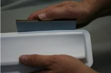
Bending at the score will break the plastic along the scored line. You can cut with scissors if you prefer. Either way, any rough edges can be smoothed out with the included 100 grit sand paper or sanding block.
