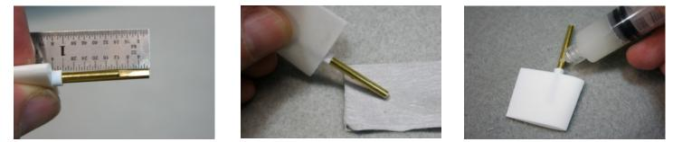
Grind a 3/8-inch flat on the leading edge of the rudder shafts facing forward. Sanding off the sharp corners of the end of the shafts will make it easier to insert into the rudder arms. Put a little grease on the shafts near the rudder blades.
