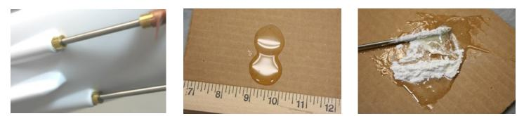
The final location for the stern tubes is with only about 1/8-inch or less protruding from the hull journals. Keep the epoxy off of the shafts. Mix two 1-1/4" puddles of epoxy and add filler.
