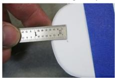
Tape the deck to the sub-deck/hull assembly. Set upright. Make a light line above each side cross-member mark. At the center of the stern (back end) make a dot 1/2 inch from the edge of the deck.
