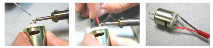
Tin the motor tabs. Connect them by holding the tinned wire to the tinned tab and apply heat to melt them together.
