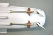
Holding each rudder straight, tighten the ez-connector screws. Connect your radio gear. Turn on your transmitter and receiver. Turn your rudders left and right. Make sure the pushrods don't contact the motor clamp at extreme left or right rudder. If they do, trim them shorter. Confirm both rudders are parallel with each other.
