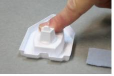
Scuff in side the line for the glue to adhere. Put CA on the bottom edge of the pilot house. Align and press in place.
