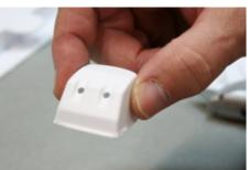
Trim the gun housings close. Then, lay the scissors along the side of each to trim closer. Once trimmed, the gun housings will still have a slight curve or flair at the bottom.
