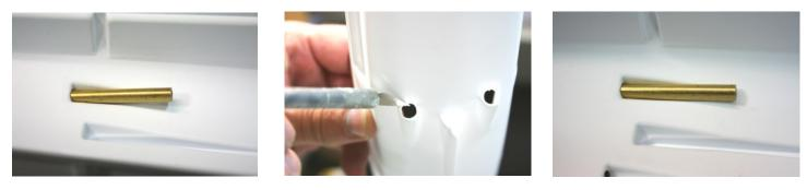
To avoid binding or excessive friction in the drive shaft, the brass stern tubes should fit fully into their hull journals (angled depressions in the hull). The hull is pre-drilled for the stern tubes, but the openings will need some adjustment if the stern tubes are up on the end when inserted like this. Once the top of the hull opening is trimmed, the stern tube will lay down into the journal.
