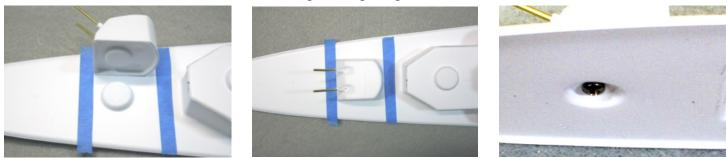
For the guns, tape will help you align the round piece under the gun with the round mount on the deck. Don't install the gun where you plan to mount your bb cannon later. After CA cures, drill 5/64" hole through deck into gun base. Insert an included #4 x 1/4" stainless screw to help hold gun in place when hit by enemy bb's to help avoid embarrassing gun loss in battle.
