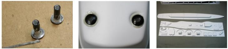
Spread epoxy on the rudder mount. Press into the hull. It should look like this. Less epoxy is OK. 7 Check the alignment and set the hull aside for the epoxy to cure. Lay out the deck and deck accessories as shown.
