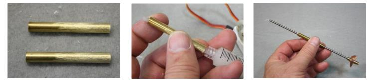
Loosen the shaft set screws and remove the motor mount and two shafts & stern tubes. Scuff the outside of the stern tubes to help them bond to epoxy. Inject grease into both stern tubes. With the sanded stern tube end pointed toward the propeller, insert a shaft into each to the shaft center which will push out excess grease. Clean off any spilled grease from the parts or on your hands. Grease will lubricate the shaft and prevent water entering the tube.
