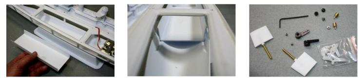
This is the electronics tray. It fits into the 2nd bay from the bow. You may not need all of it. It helps you lay out your electronics. Best to attach it later to the ballast or hull with pieces of hook & loop for easy removal for drying or working on the electronics once you have designed the layout and location of the internal parts. It holds the receiver, switches, ESC, firing boards or other components. Open the rudder package and servo packet.
