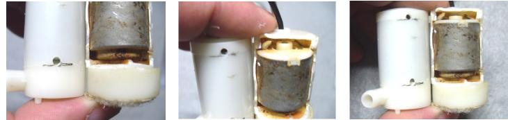
With the two holes successfully drilled, use compressed air to blow into the top hole, exhausting water out the bottom hole until no more water comes out and the interior is dry. Leave this open to dry further. Before using, cover the holes with pieces of hatch tape or dabs of hot glue. Multiple holes can be drilled at the front third of the casing. After a day of battling, remove the tape and again, blow out any water inside the unit and let it sit until dry.
