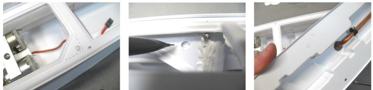
Locate and drill a 3/16 inch hole in the sub-deck as shown. If you haven't glued on the balsa skin yet, install the deck. Trace the hole on the underside of the deck and drill a 3/16 inch hole through the deck.
