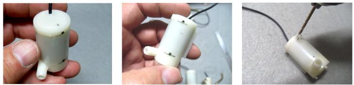
Do this just off-center to the right opposite where the wire comes out. Compare the marks to this photo showing the spaces you are drilling into. Using a 3/32 inch drill, slowly drill with light pressure preventing the drill from going further than the thickness of the white plastic casing.
