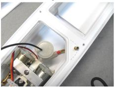
To install, from the motor compartment, hook the discharge port under the cross-member. Set the pump down, then rotate to insert the discharge port through the hole.
