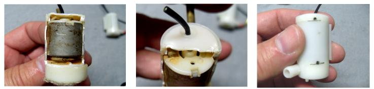
The water-resistant casing will eventually let water into the motor. On the front, opposite where the wire comes out, there are no connectors or obstructions. There is a gap above and below the motor. Mark two dots about 3/32 inches round, just above and touching the upper and lower case glue seams. (marked by the two lines)
