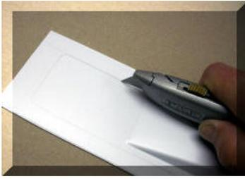
Use a box cutter or hobby knife with a new blade to score the pencil mark. Make one light pass concentrating on following the line, then follow with a second pass.
