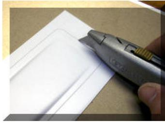
You are not cutting through the plastic. You just want to cut the surface. If you are uncomfortable with razors, then use a pair of sharp scissors to cut out the cowl
